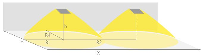
R1 distance from wall (X axis) R2 installation distance between lights (X axis) R4 distance from wall (Y axis) Y9992WA
