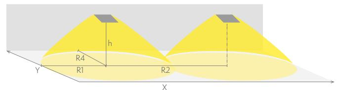
R1 distance from wall (X axis) R2 installation distance between lights (X axis) R4 distance from wall (Y axis) Y9971W
