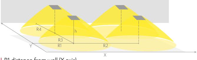
R1 distance from wall (X axis) R2 installation distance between lights (X axis) R3 installation distance between lights (Y axis) R4 distance from wall (Y axis) Y9292WMC
