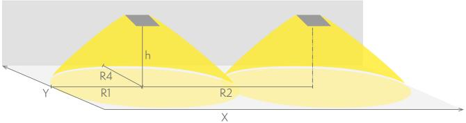
R1 distance from wall (X axis) R2 installation distance between lights (X axis)
