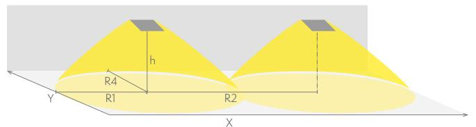
R1 distance from wall (X axis) R2 installation distance between lights (X axis) R4 distance from wall (Y axis) Y9271W
