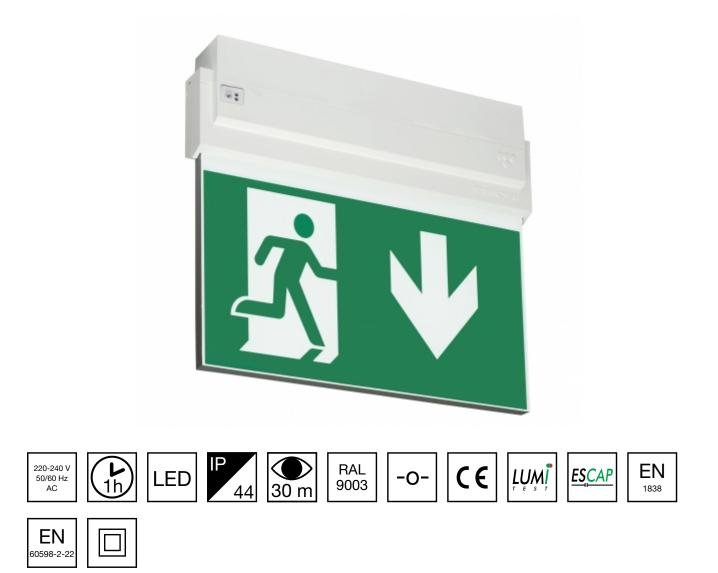
Self-contained ESCAP Emergency Exit Light with 1 h Super Capacitor and Lumi Test Self-testing with 2-sided pictogram, arrow down, 30 m viewing distance (Invidually packed TWS8092WM)
