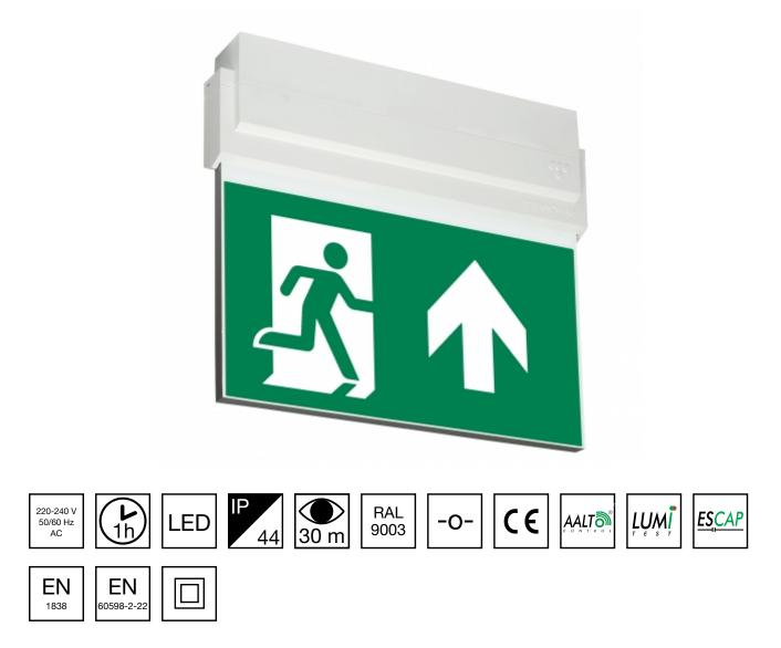
Self-contained ESCAP Emergency Exit Light with 1 h Super Capacitor and Wireless Central Monitoring, with 1-sided pictogram, arrow up, 30 m viewing distance (Invidually packed TWS8092WA)
