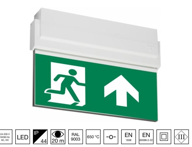
24-230 V centrally supplied LED Emergency Exit Light with 1sided pictogram, arrow up, 20 m viewing distance (Invidually packed TWT8071W)
