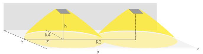
R1 distance from wall (X axis) R2 installation distance between lights (X axis) R4 distance from wall (Y axis) Y4392WA
