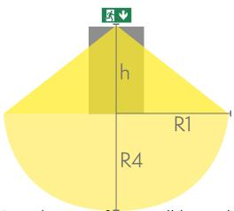
R1 distance from wall (X axis) R4 distance from wall (Y axis) Y3051WKE140
