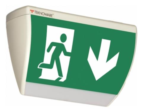
Double insulated, 24-230V centrally supplied emergency exit light with a set of pictograms, 24m viewing distance (Invidually packed TWT1771WS)
