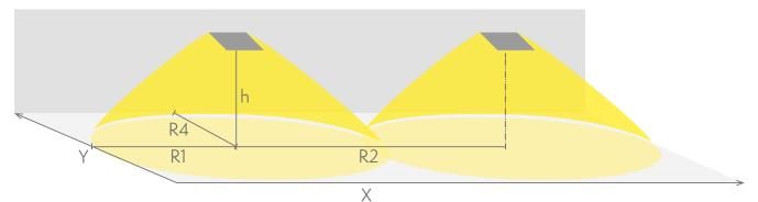
R1 distance from wall (X axis) R2 installation distance between lights (X axis) R4 distance from wall (Y axis) TWTC152WM
