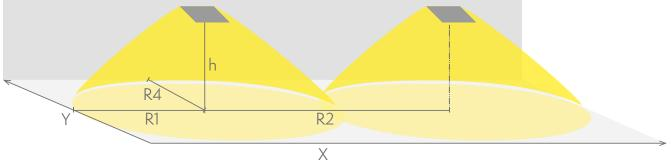
R1 distance from wall (X axis) R2 installation distance between lights (X axis) R4 distance from wall (Y axis) TWT9252WM
