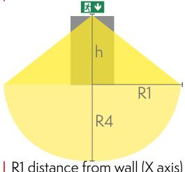
R1 distance from wall (X axis) R4 distance from wall (Y axis) TWT9051WK
