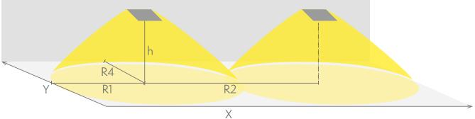
R1 distance from wall (X axis) R2 installation distance between lights (X axis) R4 distance from wall (Y axis) TWT4371W
