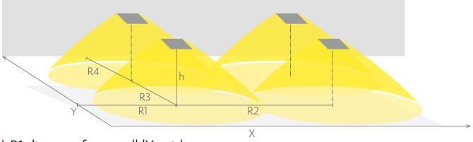
R1 distance from wall (X axis) R2 installation distance between lights (X axis) R3 installation distance between lights (Y axis) R4 distance from wall (Y axis) TWT3252WM
