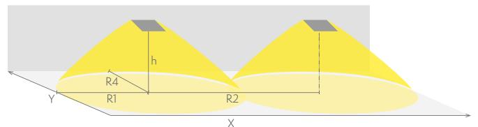
R1 distance from wall (X axis) R2 installation distance between lights (X axis) R4 distance from wall (Y axis) TWS9992WMT
