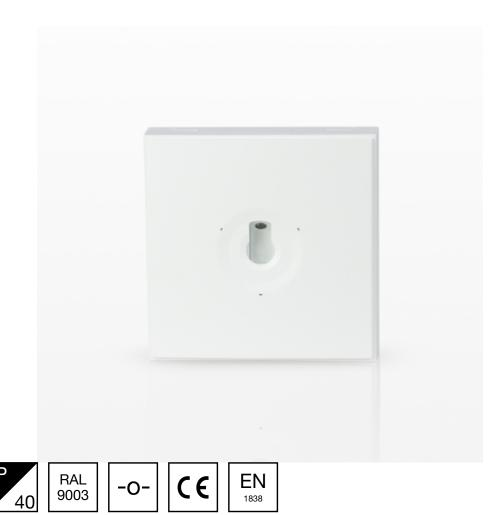
Teknoware Zonespot II Angle is a surface-mounted emergency light that illuminates safety equipment, such as fire alarm call points, first aid stations, firefighting equipment and panels, vertically with 5 lux according to EN 1838. Zonespot II Angle has been designed for indoor lighting, and the standard colour is white (RAL 9003). Installation is quick and easy, with a separate mounting base that also handles the power supply connection.
