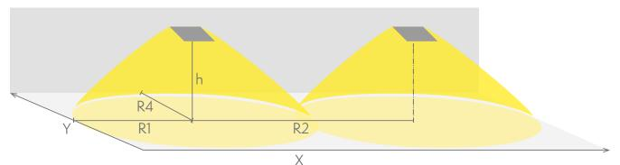
R1 distance from wall (X axis) R2 installation distance between lights (X axis) R4 distance from wall (Y axis) YB153WM120
