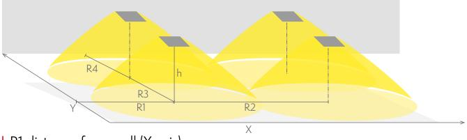
R1 distance from wall (X axis) R2 installation distance between lights (X axis) R3 installation distance between lights (Y axis) R4 distance from wall (Y axis)
