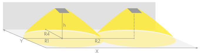
R1 distance from wall (X axis) R2 installation distance between lights (X axis) R4 distance from wall (Y axis) Y9253WM
