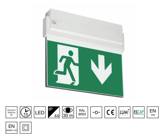
Self-contained ESCAP Emergency Exit Light with 1 h Super Capacitor and Lumi Test Self-testing with 1-sided pictogram, arrow down, 30 m viewing distance (Invidually packed TWS8092WM)
