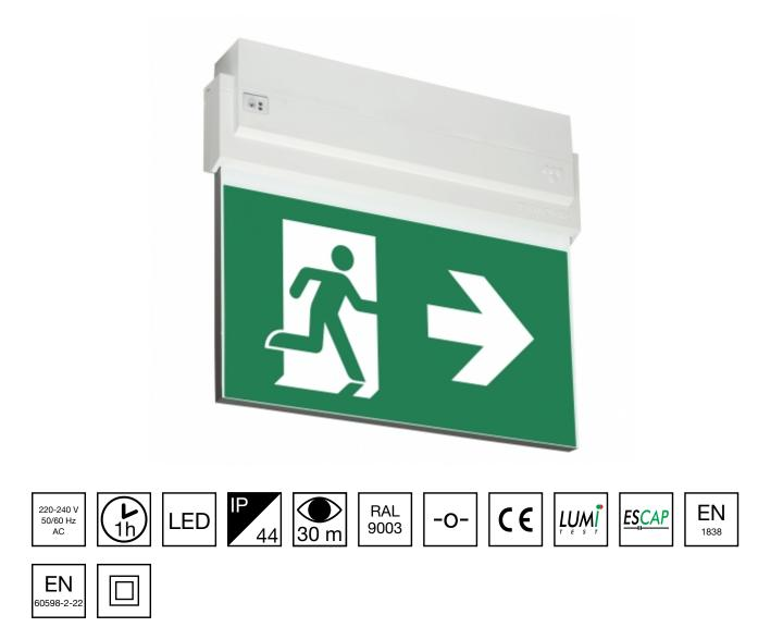
Self-contained ESCAP Emergency Exit Light with 1 h Super Capacitor and Lumi Test Self-testing with 1-sided pictogram, arrow right, 30 m viewing distance (Invidually packed TWS8092WM)
