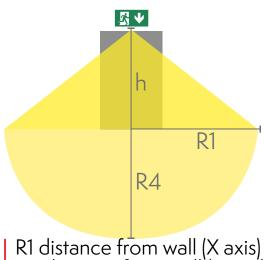
R1 distance from wall (X axis) R4 distance from wall (Y axis) Y8051WK108
