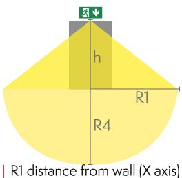
R1 distance from wall (X axis) R4 distance from wall (Y axis) Y8051W148
