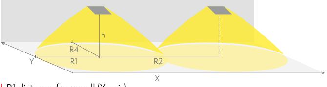
R1 distance from wall (X axis) R2 installation distance between lights (X axis) R4 distance from wall (Y axis) TWTB153WM
