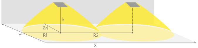
R1 distance from wall (X axis) R2 installation distance between lights (X axis) R4 distance from wall (Y axis) TWT9951WK
