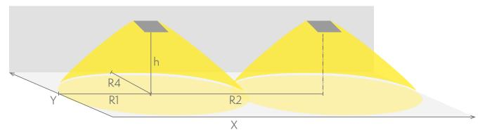
R1 distance from wall (X axis) R2 installation distance between lights (X axis) R4 distance from wall (Y axis) TWT6171W
