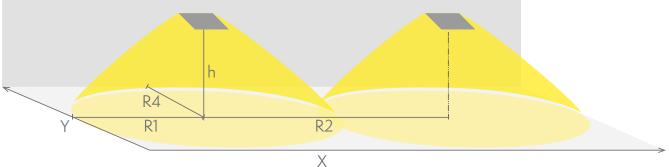
R1 distance from wall (X axis) R2 installation distance between lights (X axis) R4 distance from wall (Y axis) TWT4352WM
