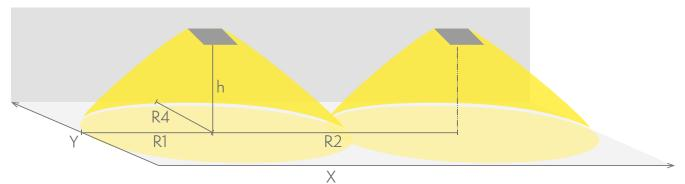
R1 distance from wall (X axis) R2 installation distance between lights (X axis) R4 distance from wall (Y axis) TWSC292WA
