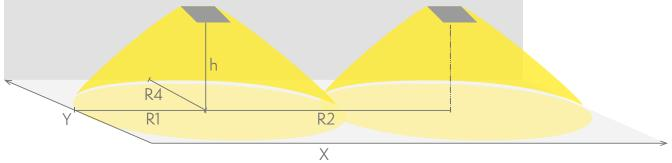
R1 distance from wall (X axis) R2 installation distance between lights (X axis) R4 distance from wall (Y axis) TWS9992WM
