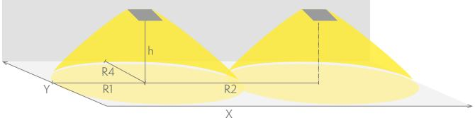
R1 distance from wall (X axis) R2 installation distance between lights (X axis) R4 distance from wall (Y axis) TWS4392WA
