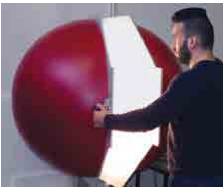
We use the Ulbricht sphere for the measurement of the luminous flux of luminaires in our lighting laboratory.
