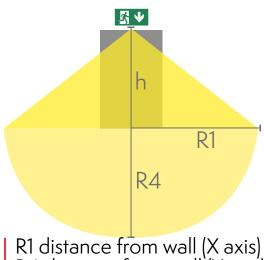
R1 distance from wall (X axis) R4 distance from wall (Y axis) Y8051WK103
